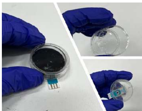
Figure 1. SPCE/Petri Dish Production: A 7 mm 2 CNC-machined window was opened at the bottom of the petri dish and attached to the bottom using SPCE (DRP-110) non-toxic adhesive. For the sealing test, colored liquid was used and kept for 24 hours.
