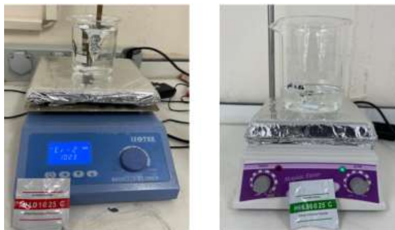
Figure 11. Experimental setup for buffered impregnation media prepared in distilled water and conditioned to chemical equilibrium
