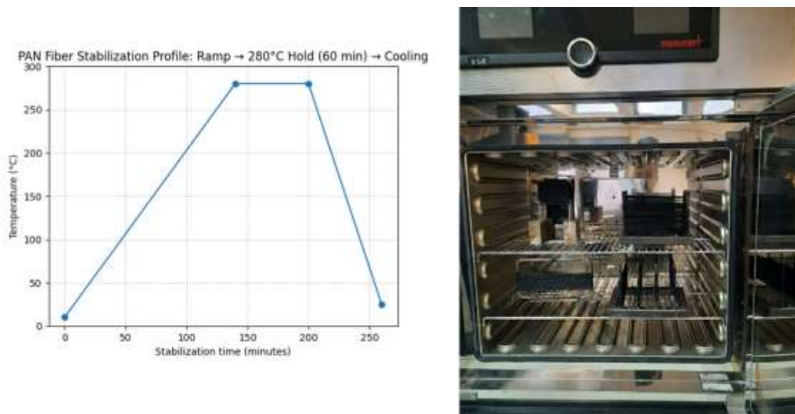
Figure 14. Single ramp PAN fiber stabilization at 280°C (60 min) and cooling, with the drying oven
