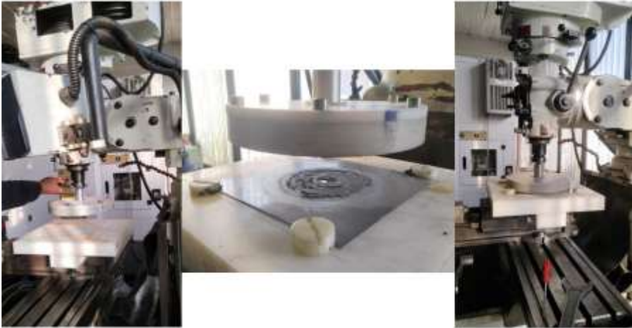
Figure 1. Experimental setup for the Magnetic Abrasive Finishing (MAF) tests on flat surfaces
