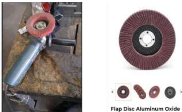
Figure 5. Polishing device and abrasive disc
